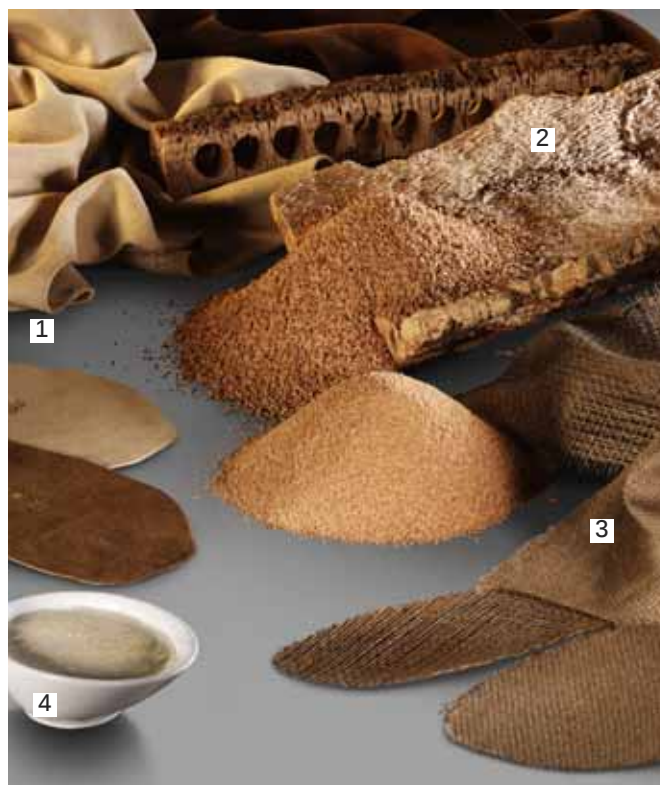
Suede leather in one piece and stamped (1), cork bark, stamping residue and granulate (2), fine and coarse jute (3) and latex milk (4) – natural materials for our footbed.
